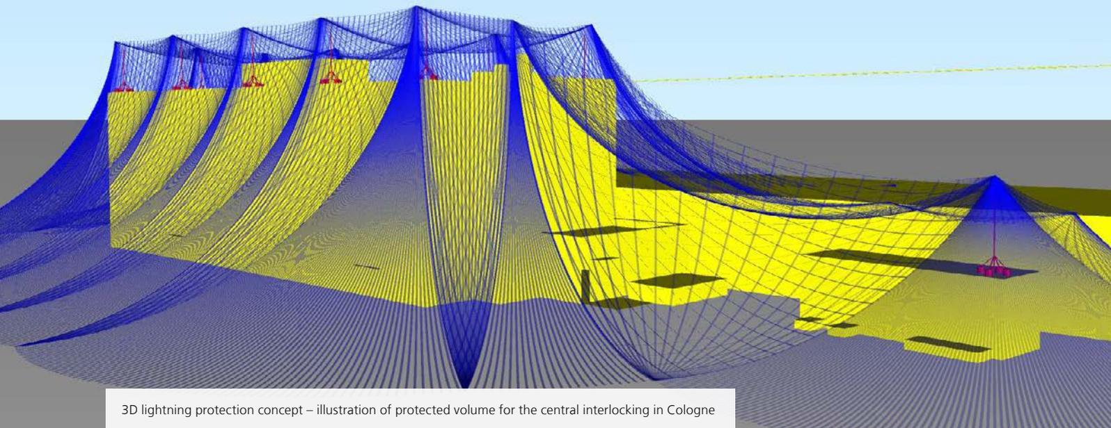
3D lightning protection concept – illustration of protected volume for the central interlocking in Cologne
