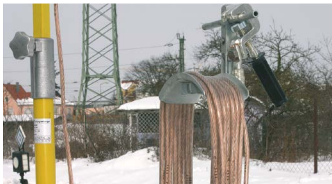
Earthing spike with coiled earthing cable.
