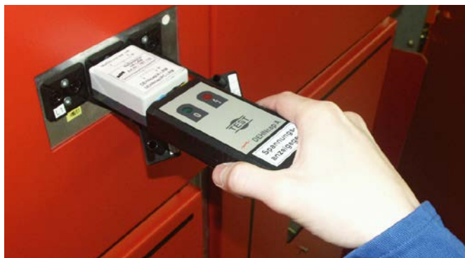
Self-test of a DEHNCap/A voltage indicator.
