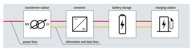
In public spaces, powerful charging parks (HPC: high-power charging) or bus depots are electrified. Therefore, additional transformer stations, converter units, battery storage systems and, ultimately, DC-supplied charging stations are set up. If just one part of the charging infrastructure is damaged by a surge, the availability of the entire charging park disappears.
